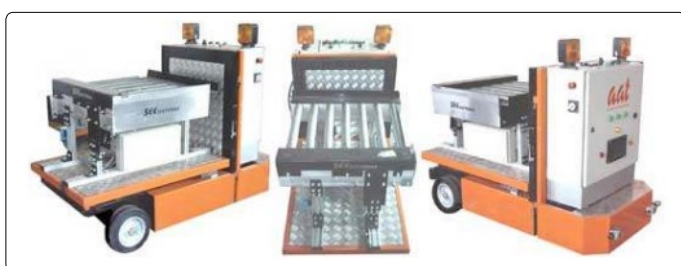
Figure 15. Automated guided vehicle (AGV).
