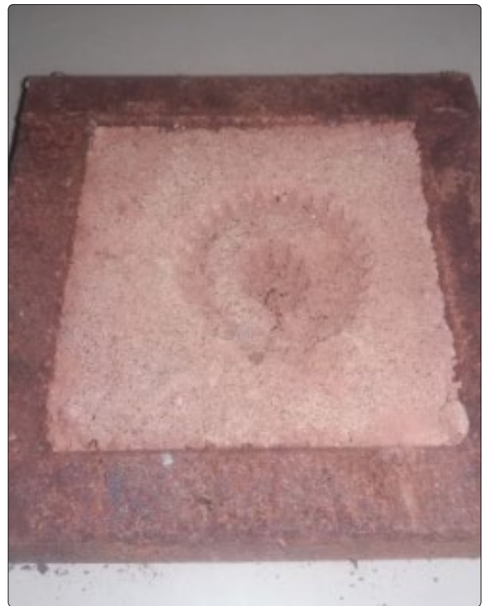
Figure 8. Sand mold for the first gear.
