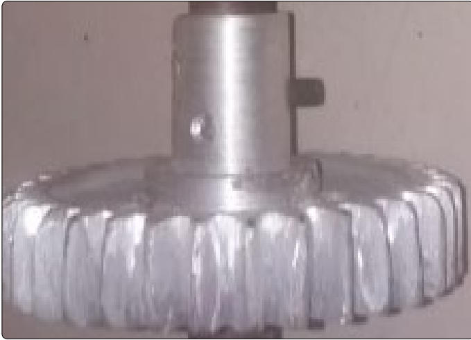
Figure 10. Gear 4 as cast.
