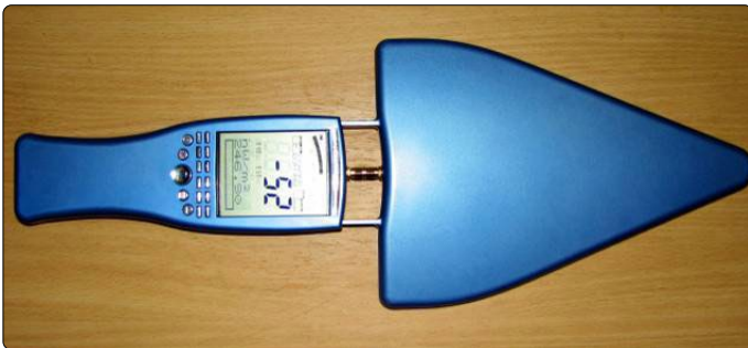
Figure 1. The spectrum analyzer connected with the antenna via SMA adapter.
