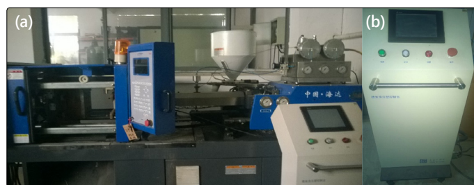
Figure 4. Microcellular foam injection molding device: (a) injection machine, (b) microcellular foam console.
