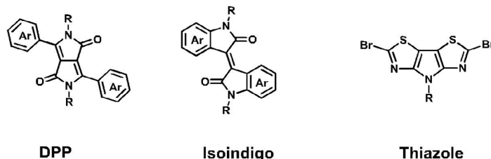
Figure 1- Chemical structures of DPP, Isoindigo and bis-thiazole.
