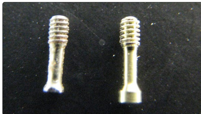
Figure 7. A main screw fractured under overload and/or excessive tightening with its intact original.
