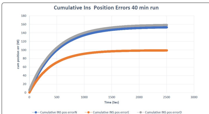
Figure 12. Cumulative INS position errors for 40 min period.
