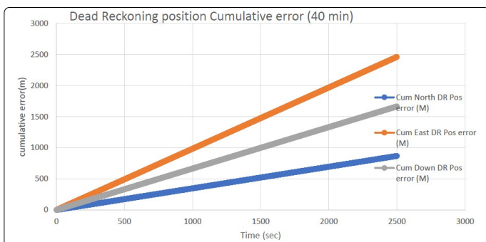
Figure 14. Dead Reckoning cumulative position error (40 min).
