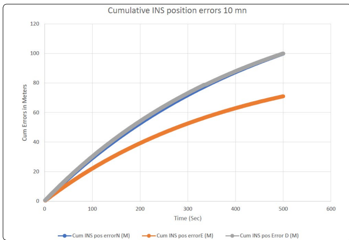
Figure 10. Cumulative INS position errors for 10 min period.
