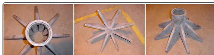
Figure 2. Multi arm flare burner tip (courtesy of Zeeco, Inc.)
