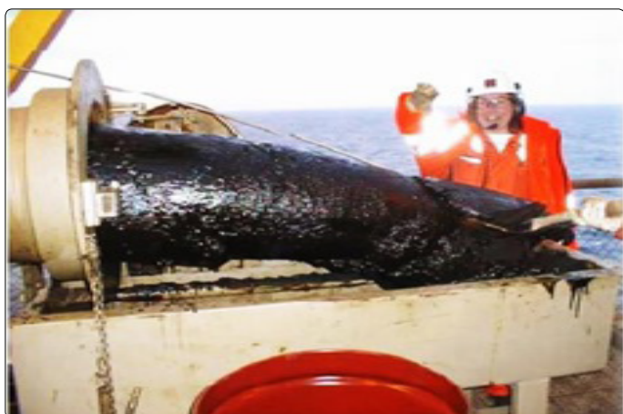
Figure 2. Wax deposition plug in the wellbore on platform C in the North Sea [19].
