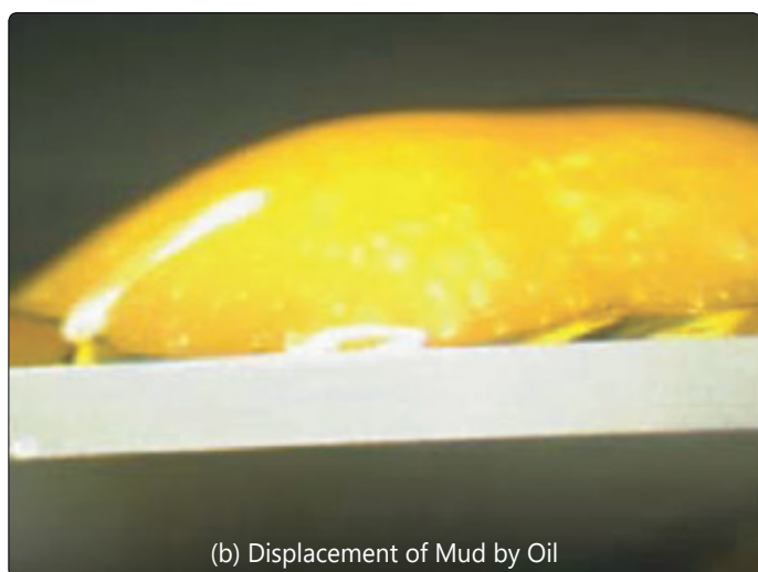
Fig 4. APHRON drilling fluids and crude oils are very compatible as shown by the low contact angles [43].
